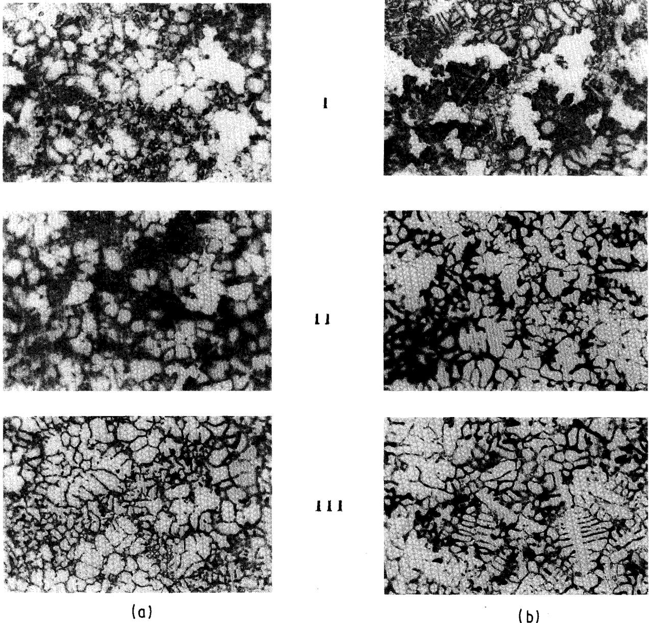
Figure 12 Typical microstructure obtained in stir-cast Pb-6Sb alloy cast at a temperature in the mushy zone (265 °C) in three different steel moulds: (I) 18 mm, (II) 25 mm and (III) 32 mm diameter for speeds of (a) 1100 and (b) 400 r.p.m. (50 ×).
