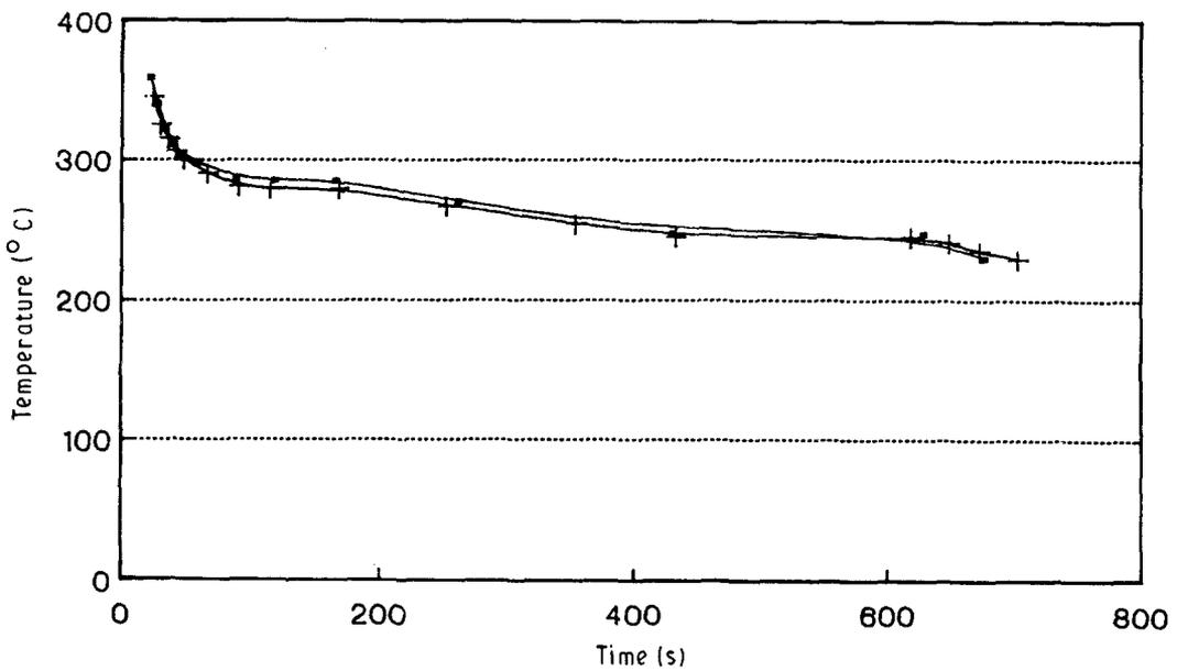
Figure 6 Cooling curves of Pb-6Sb alloy conventionally cast in a 40 mm inner diameter steel mould, (+) with addition of 0.02% Ag<sub>2</sub>Se grain refiner (GR) and (■) without addition (CC).
