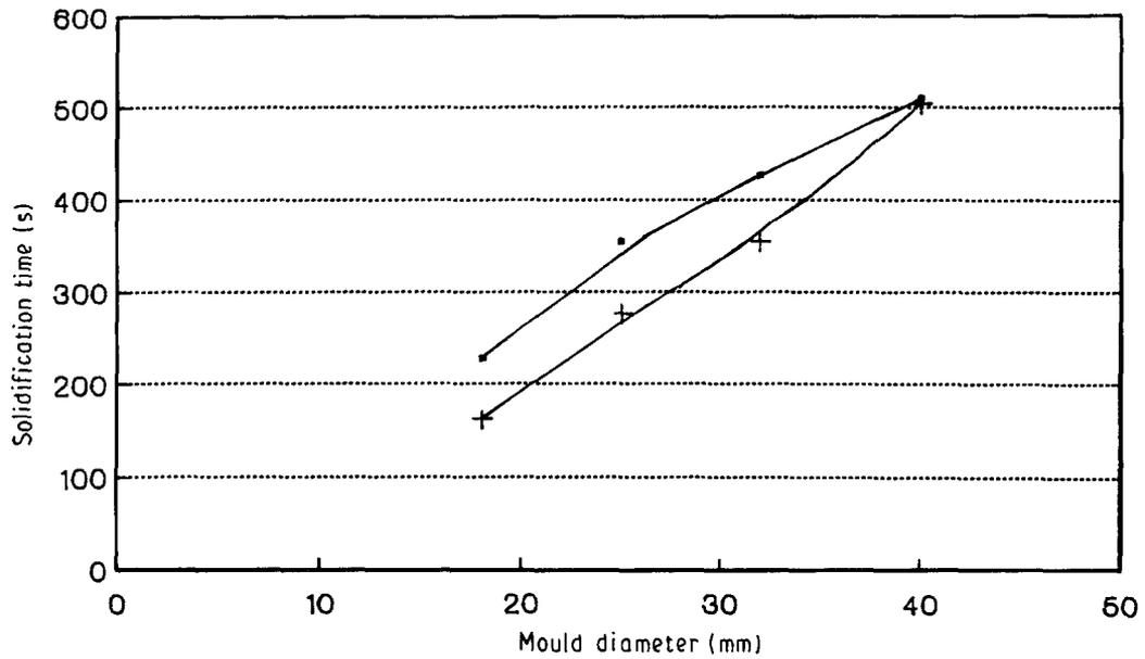
Figure 7 Influence of mould diameter on the solidification time of (■) conventionally cast (CC) and (+) grain-refined (GR) alloy.
