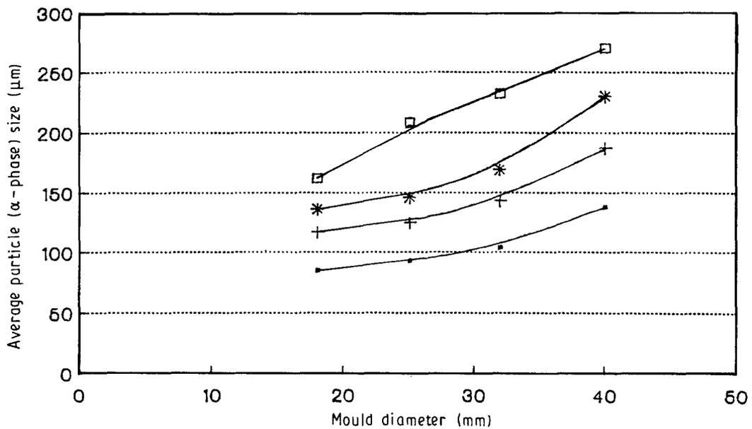
Figure 13 Effect of mould diameter on the average particle ( $\alpha$ -phase) size of Pb-6Sb alloy stirred at four different stirring speeds: (□) 400, (\*) 700, (+) 900 and (■) 1100 r.p.m.
