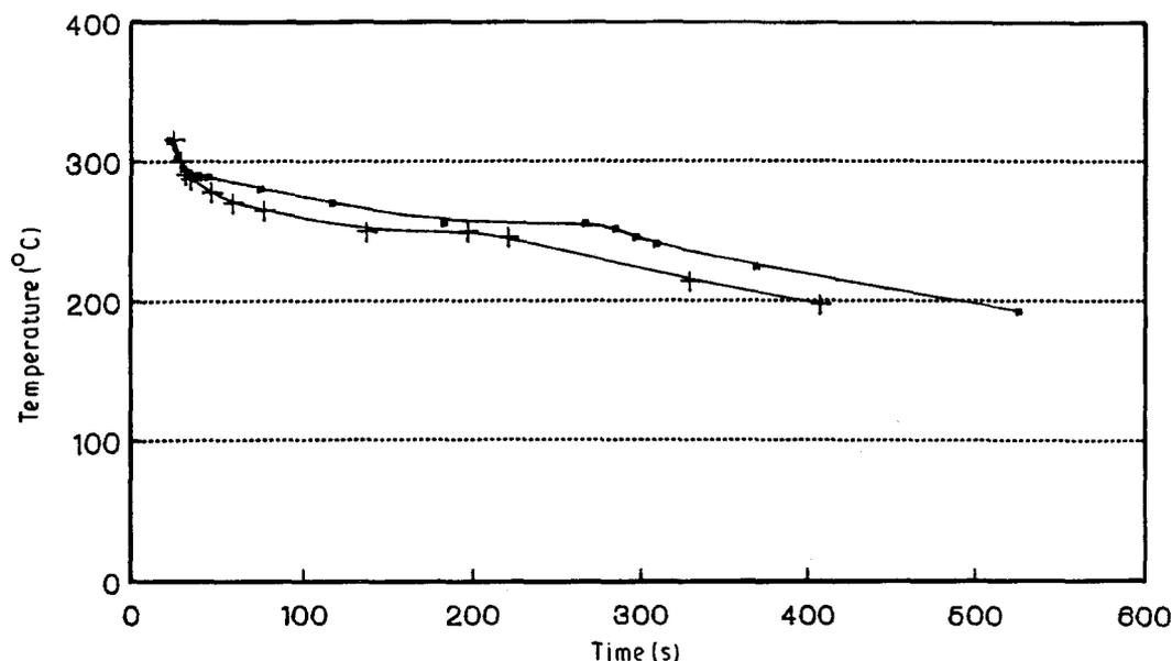
Figure 3 Cooling curves of Pb-6Sb alloy conventionally cast in an 18 mm inner diameter steel mould, (+) with addition of 0.02% Ag<sub>2</sub>Se grain refiner (Gr) and (■) without addition (CC).
