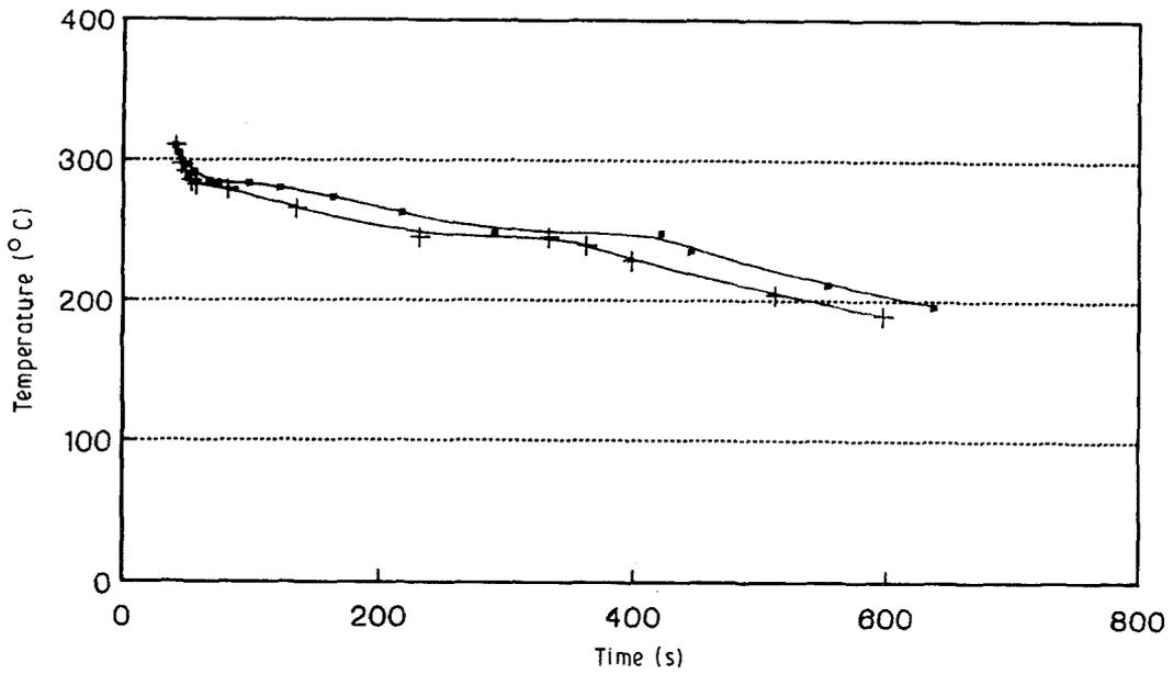
Figure 4 Cooling curves of Pb-6Sb alloy conventionally cast in a 25 mm inner diameter steel mould, (+) with addition of 0.02% Ag<sub>2</sub>Se grain refiner (GR) and (■) without addition (CC).
