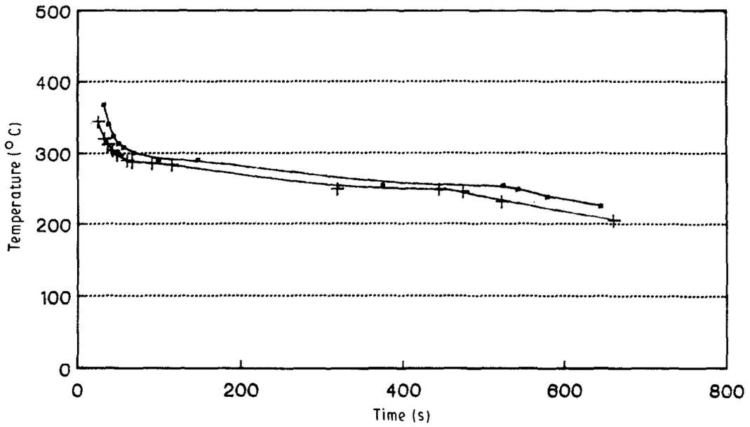
Figure 5 Cooling curves of Pb-6Sb alloy conventionally cast in a 32 mm inner diameter steel mould, (+) with addition of 0.02% Ag<sub>2</sub>Se grain refiner (Gr) and (■) without addition (CC).
