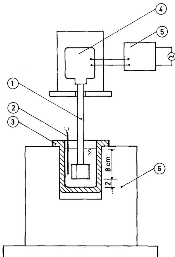
Figure 2 Schematic drawing of the stirring apparatus: (1) steel stirrer, (2) thermocouple, (3) steel crucible, (4) variable-speed motor, (5) speed control unit, (6) refractory material.
