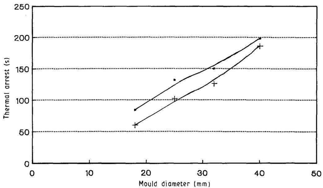
Figure 8 Influence of mould diameter on the thermal arrest of (■) conventionally cast (CC) and (+) grain-refined (GR) alloy.
