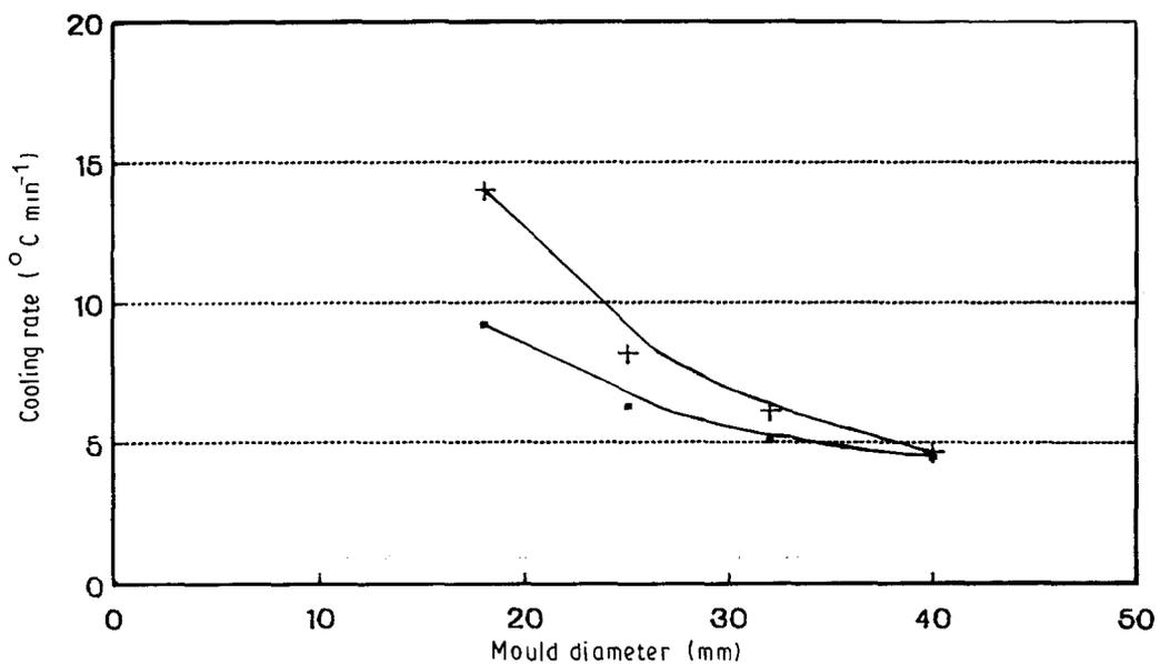
Figure 9 Average cooling rate of (■) conventionally cast (CC) and (+) grain-refined (GR) alloy as function of mould diameter.
