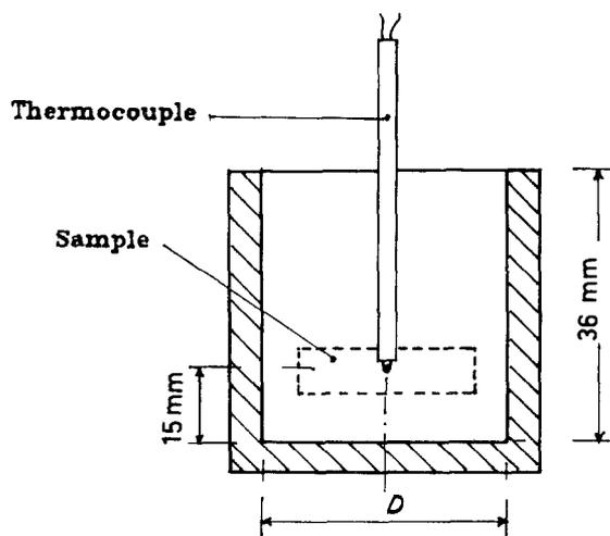
Figure 1 Level of thermocouple and microstructure sample in the steel mould of four different diameters ( $D$ ) of 18, 25, 32 and 40 mm.
