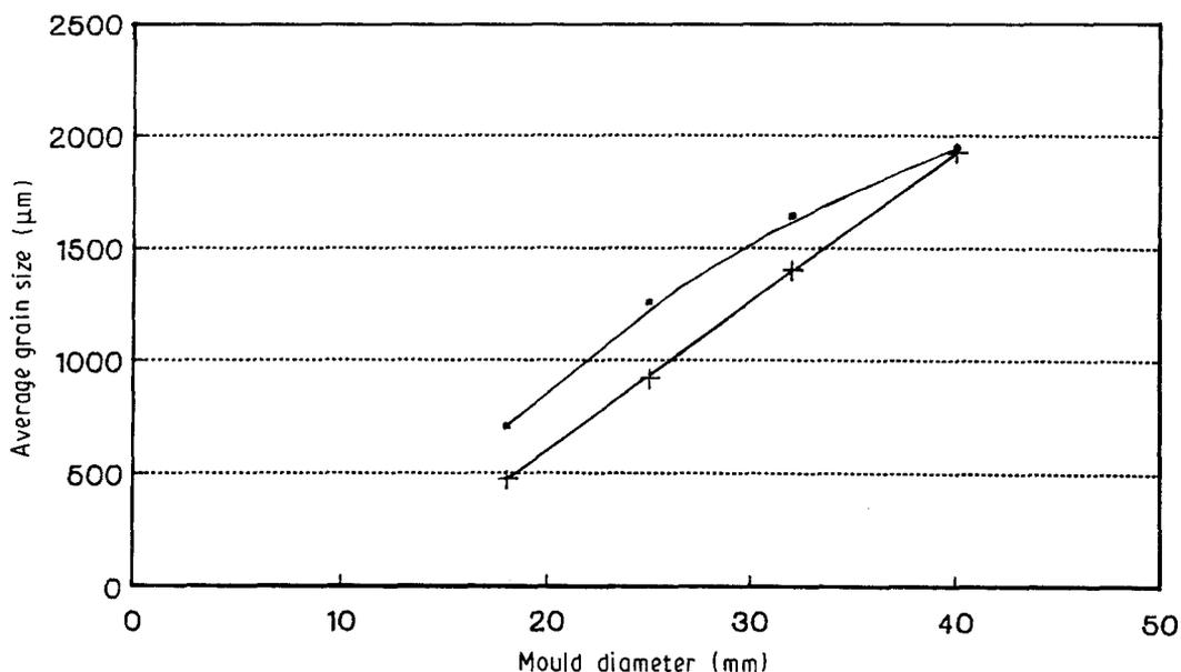
Figure 10 Average grain size of the alloy solidified (■) without addition (CC) and (+) with addition of the grain refiner (GR).
